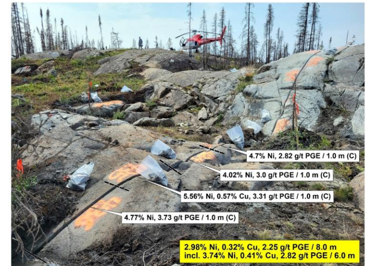
Photo 1 - Channel 1 (view to the southwest) : total horizontal length of 12.0 m, 1-m long channel samples, results of 4 samples reported on this picture.
