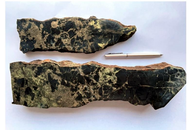
Photo 2 - Semi-massive mineralization with pentlandite, chalcopyrite and pyrrhotite in brecciated ultramafic volcanics. Sample G435309 : 9.35% Ni, 1.10% Cu, 0.147% Co, 0.29 g/t Pt, 2.11 g/t Pd
