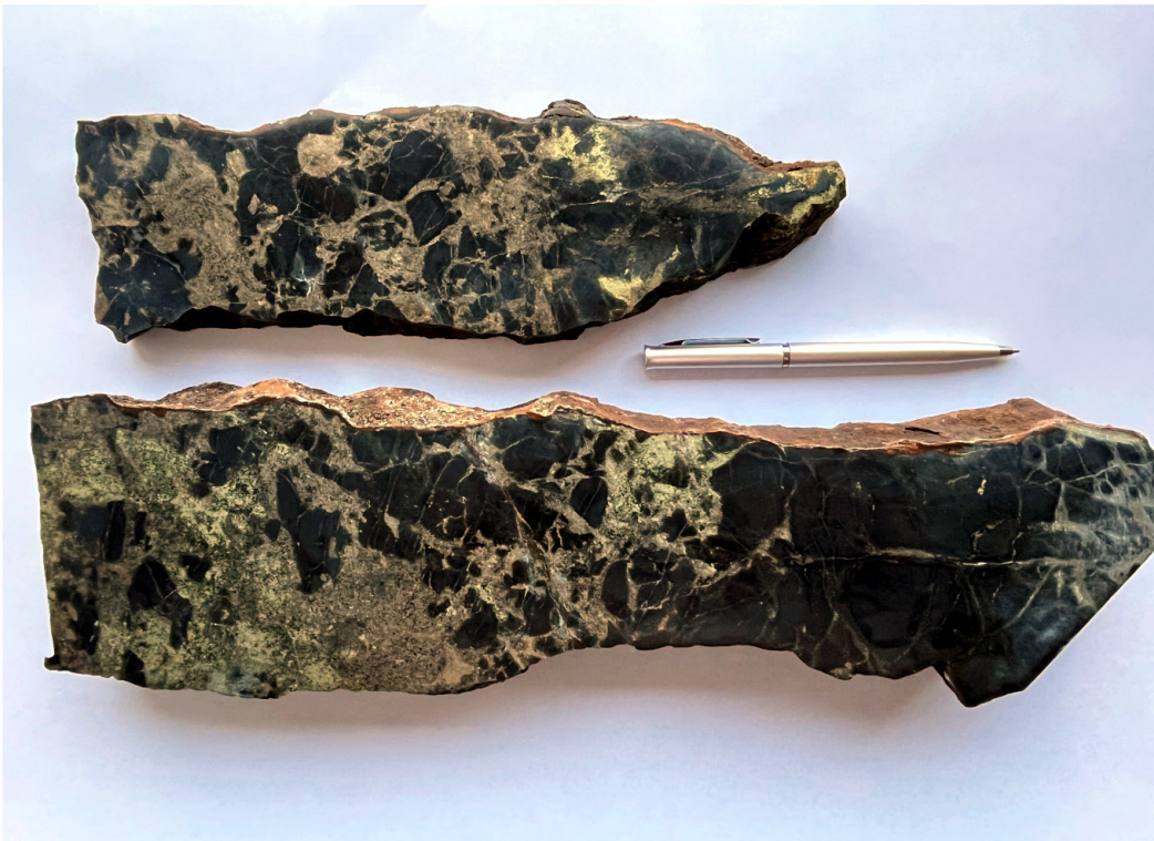
Photo 2 - Semi-massive mineralization with pentlandite, chalcopyrite and pyrrhotite in brecciated ultramafic volcanics. Sample G435309 : 9.35% Ni, 1.10% Cu, 0.147% Co, 0.29 g/t Pt, 2.11 g/t Pd
