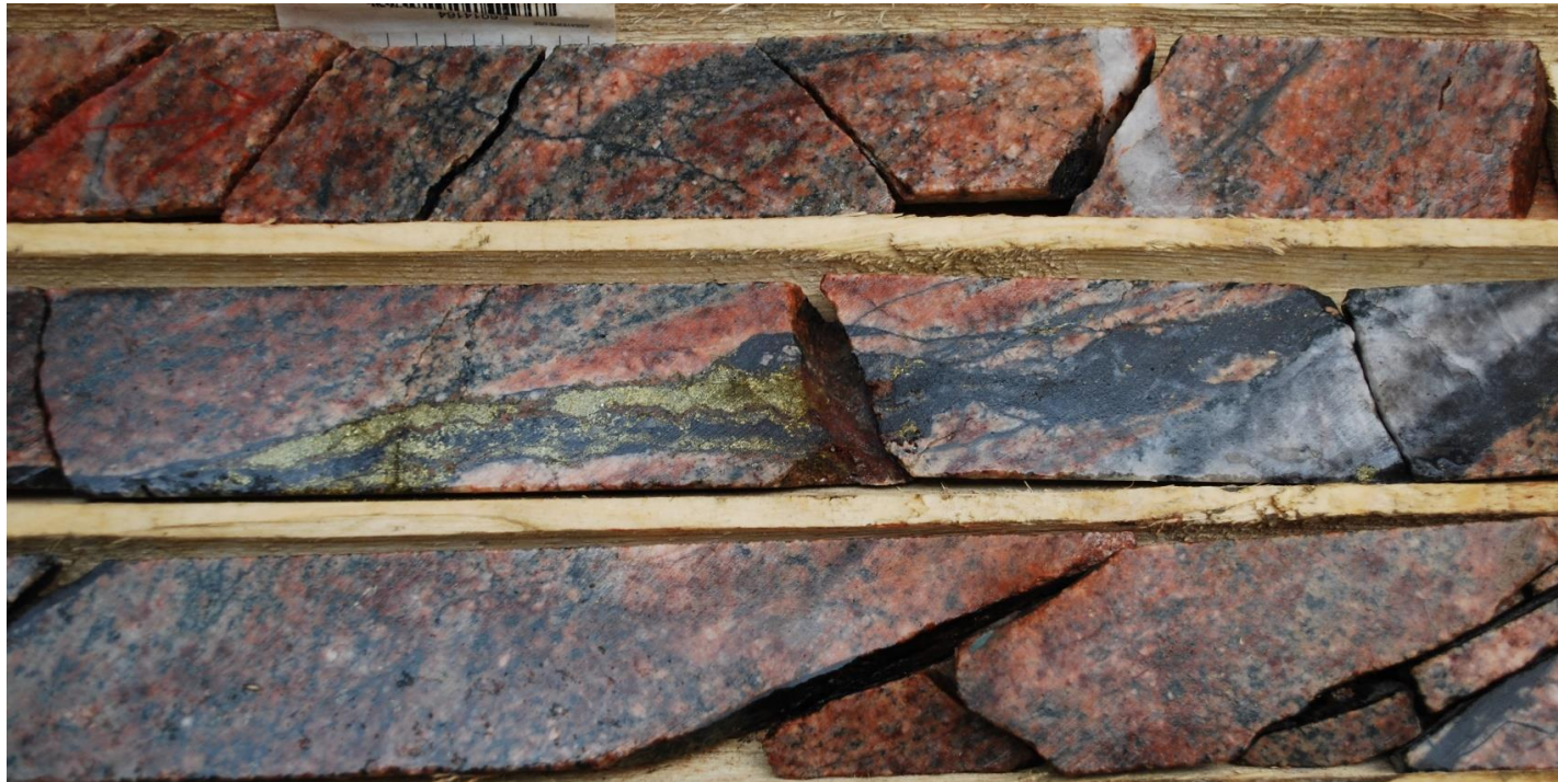
Hole Rex21-008 – Box 29 (chalcopyrite veinlet at ~127.0 m along hole)
