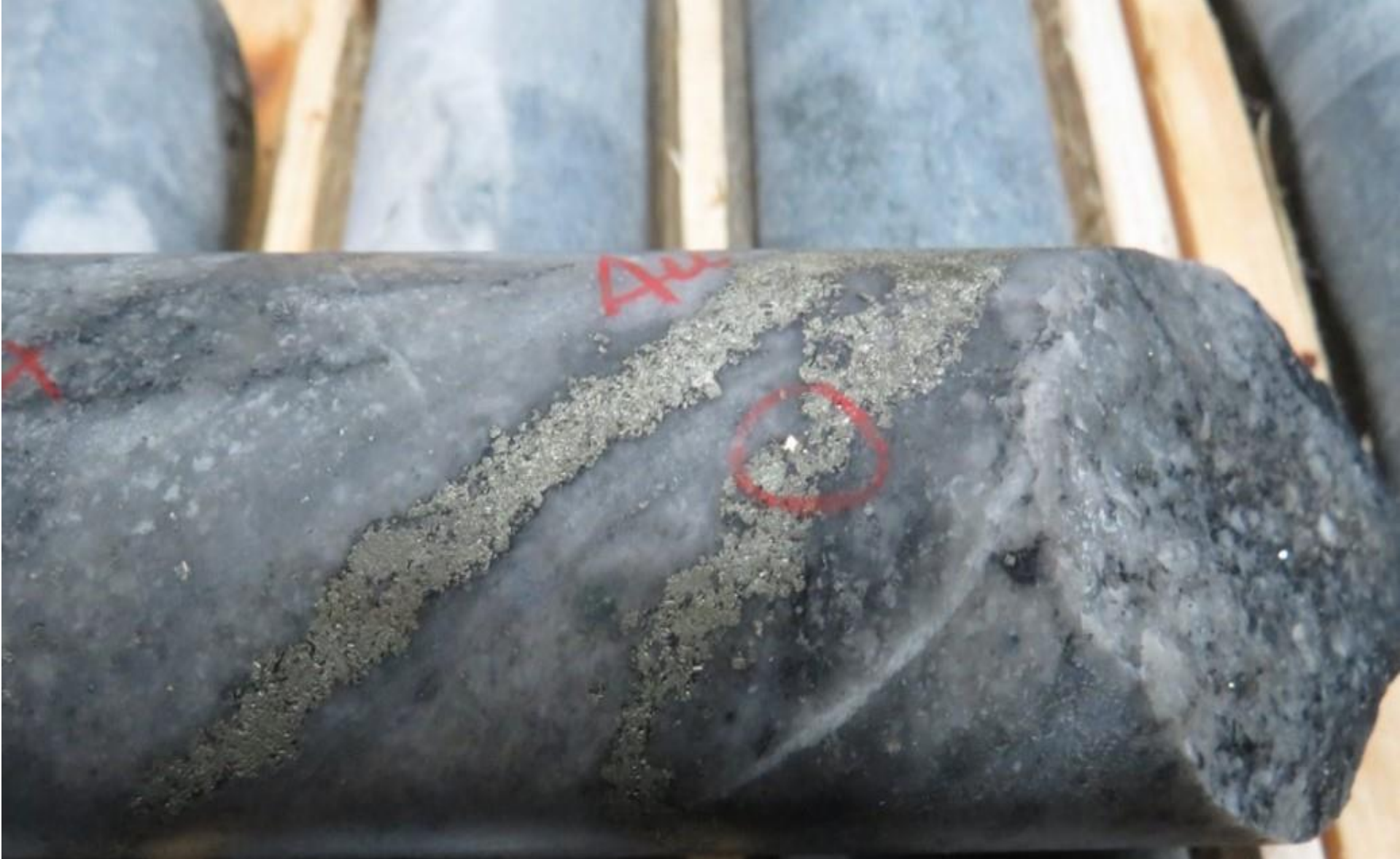
Hole ELM19-006: Native gold in a pyritic stringer in felsic intrusion at 70.7 m 121.0 g/t Au over 0.50 m
