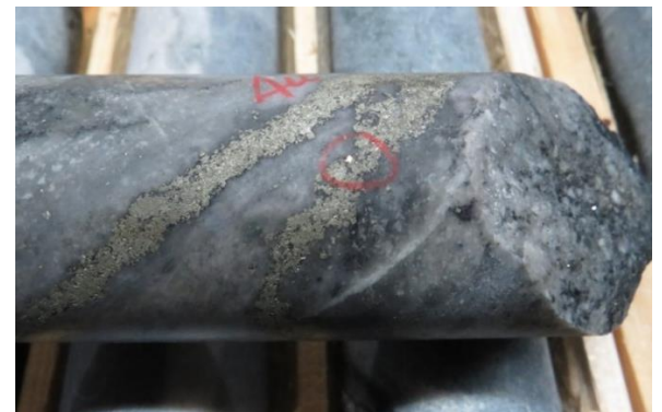
Hole ELM19-006: Native gold grain in a pyritic stringer in felsic intrusion at 70.7 m
