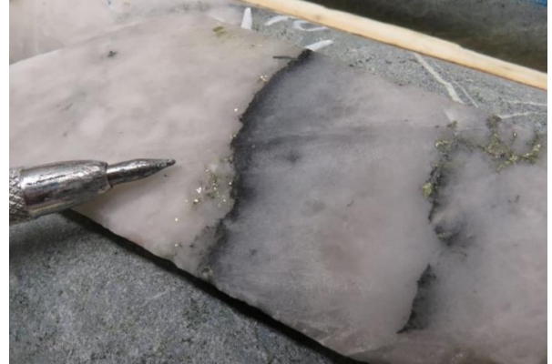
Hole ELM19-004: Native gold in milky quartz vein with tourmaline selvages at 16.2 m
