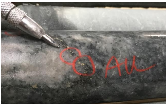
Hole ELM19-006: Native gold in a quartz chlorite vein hosted by a porphyritic felsic intrusion at 104.7 m
