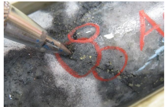
Hole ELM19-005: Native gold in a thin chloritic veinlet at 104.7 m with 1% to 3% pyrite and sericite-silica alteration
