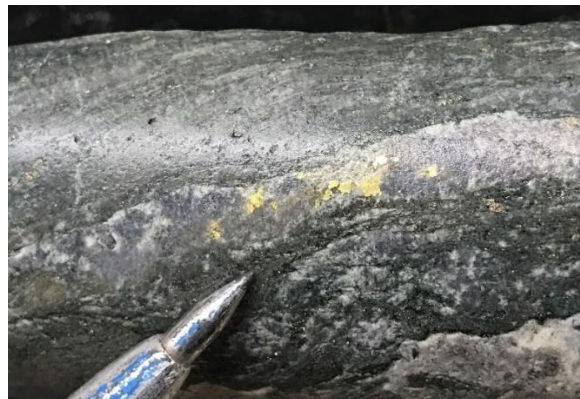
Hole ELM19-003: Native gold in quartz-carbonate veinlet subparallel to schistosity at 34.6 m
