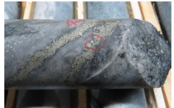
Hole ELM19-006: Native gold grain in a pyritic stringer in felsic intrusion at 70.7 m
