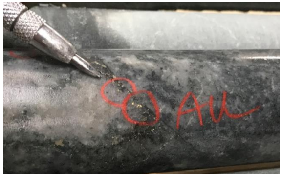
Hole ELM19-006: Native gold in a quartz chlorite vein hosted by a porphyritic felsic intrusion at 104.7 m
